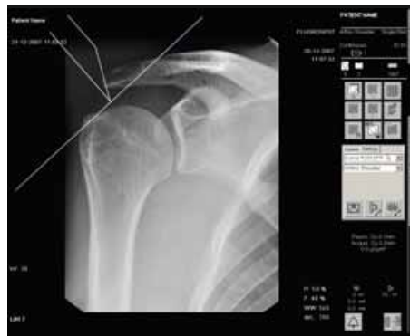
CAREPROFILE: radiation-free collimation via graphic display of the collimator and semitransparent filter position
