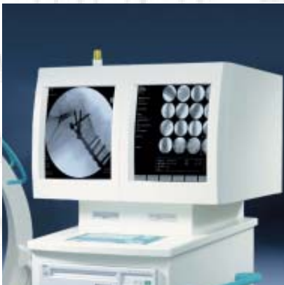
16 image mosaic is used to search the cases stored in the image memory.
